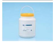
This gasket paste is suitable for use with oil-type fluids. It consists of fine mica powder blended with a water-soluble binder which is highly resistant to oil and solvents.
